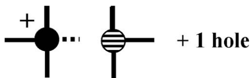
Fig. 8. The bonding associated with substituting a boron atom for an atom of a group V element in the B_{12}X_2 -type icosahedral-boride insulators is schematically depicted. The horizontally striped and solid circles denote the boron and the group V atoms, respectively. The solid lines depict two-electron bonds. The dashed line indicates a singly occupied orbital. Each boron atom substituted for an atom of a group V element introduces a hole among icosahedral internal-bonding orbitals.
